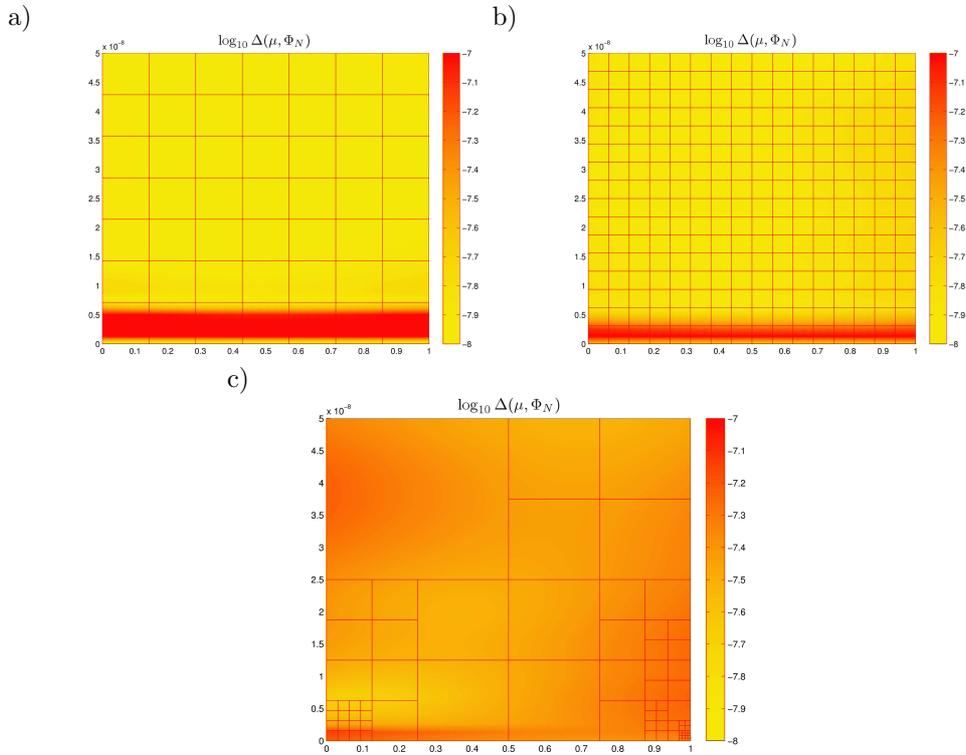
Figure 5: Demonstration of the overfitting phenomenon for a basis of size  $N = 130$  in two-dimensional parameter space  $\boldsymbol{\mu} = (\beta, \delta) \in \mathcal{P} = [0, 1] \times [0, 5 \cdot 10^{-8}]$  with a) the uniform-fixed, b) the uniform-refined and c) the local adaptive-refined grid approach.
