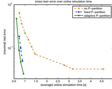
Figure 8: Comparison of different basis generation approaches regarding the maximal test error on the domain versus final (average) online-simulation time.
