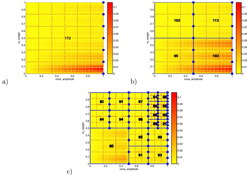
Figure 7: Demonstration of different basis generation approaches using the standard (POD-)greedy procedure on each subdomain. The colors indicate the test error over the parameter domain. a) No parameter domain partition ( $\varepsilon < \varepsilon_{tol}, N$  very large), b) uniform parameter domain partition ( $\varepsilon \leq \varepsilon_{tol}, N$  large), c) adaptive parameter domain partition ( $\varepsilon \leq \varepsilon_{tol}, N \leq N_{max}$ ).
