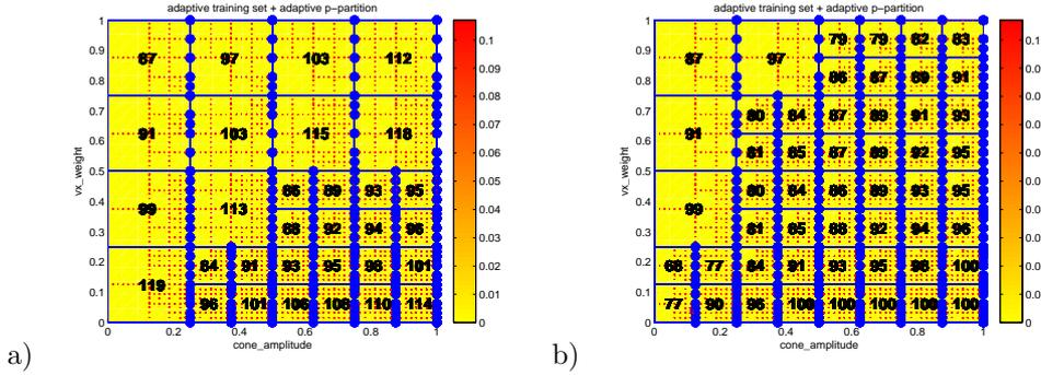
Figure 9: Demonstration of the adaptive parameter domain partition approach using the local adaptive training set extension method on each sub-domain. In a) the basis size was limited to  $N_{max} = 120$  and in b) the limit was  $N_{max} = 100$ . We see that for the same training error of  $\varepsilon_{tol} = 0.0001$  a smaller basis size limit leads to a finer partition of the parameter domain.
