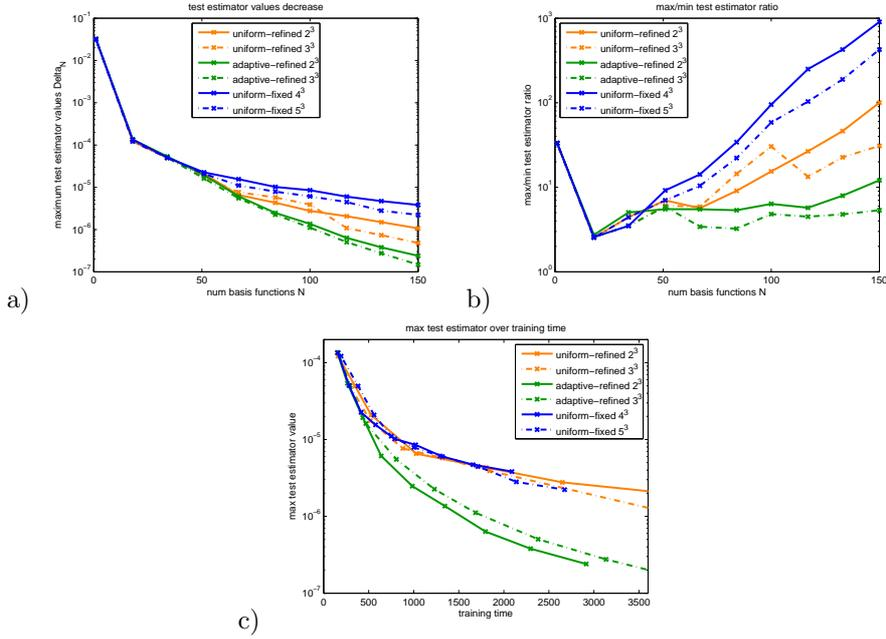
Figure 6: Quantitative comparison of the basis-generation approaches with respect to a) maximum test error, b) ratio of maximum to minimum test error and c) maximum test error over training time.
