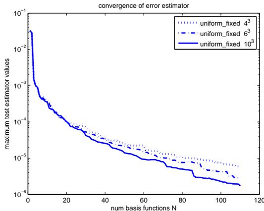
Figure 1: Illustration of overfitting for the model from [10]. The maximum error estimator on a random test set is plotted over the dimension  $N$  of the reduced basis space for the *POD-greedy* algorithm with a fixed training set corresponding to the vertices of a uniform Cartesian parameter grid with  $4^3$ ,  $6^3$ , and  $10^3$  nodes.
